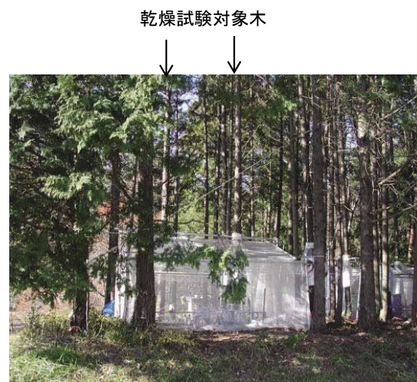
Photo 1. 降雨遮断の様子 (ヒノキ砂質壤土乾燥区) A drought experiment via rainfall interception (hinoki sandy loam drought plot)
