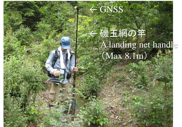
電波が弱い樹冠下でのGNSS(GPS)測量 GNSS survey under forest canopy using a landing net handle.
