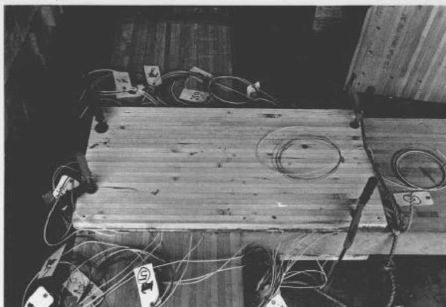
Photo. 9 Glulam moment resisting T-shape joint specimen composed of nails with steel side plates. A glulam plate of 30 mm thickness was glued on the steel side plate to protect it from direct fire attack in the fire endurance test. This experiment is being done with co-operation with Fire Protection Research Laboratory (CN43-38KAWA-17).
