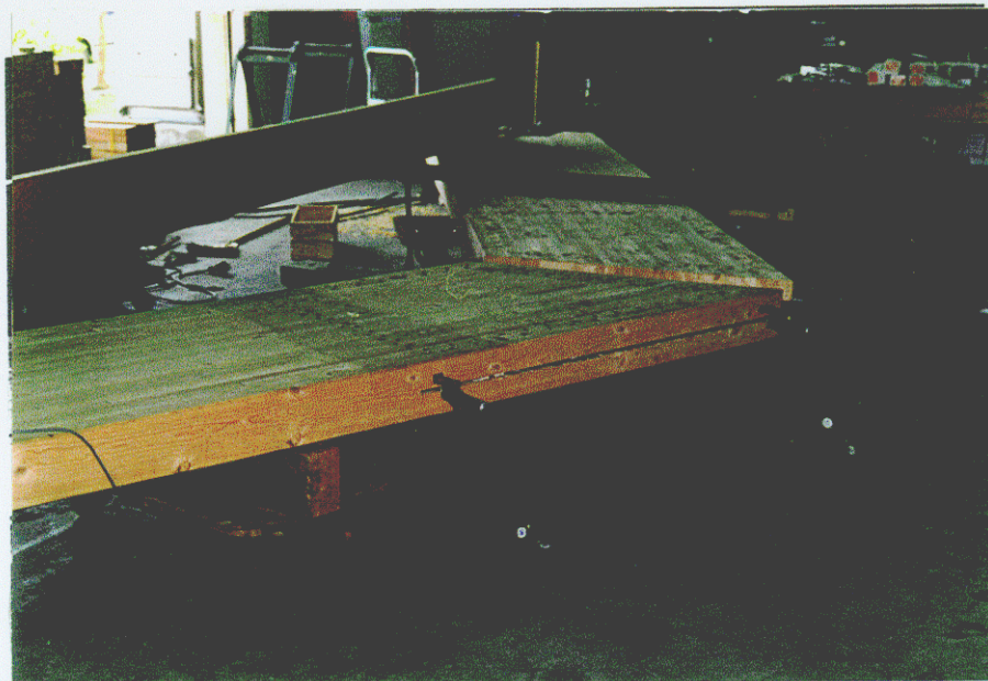
Photo. 11 Static cyclic loading test on glulam knee joint specimen. This joint is basically composed of drift pin joint with insert steel plate, but steel plate itself is also connected on-site by the "high-tension bolts" to make the on-site labor easier than the conventional method (CN1090-19).
