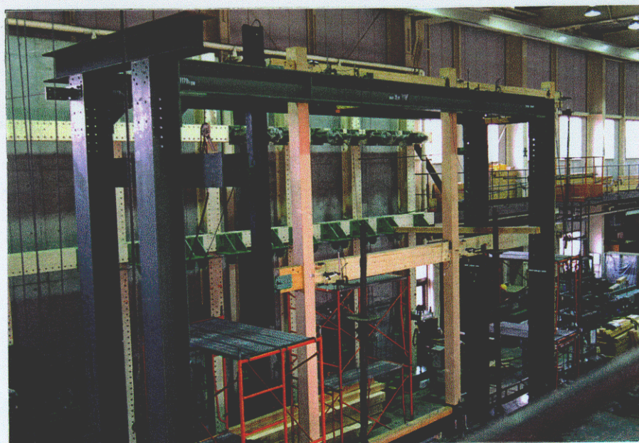
Photo. 13 Static cyclic horizontal loading test on a full-size two story post and beam frame structure. Post and beam joint was basically composed of traditional splint tenon with hardwood dowels joint (CN9156-32).
