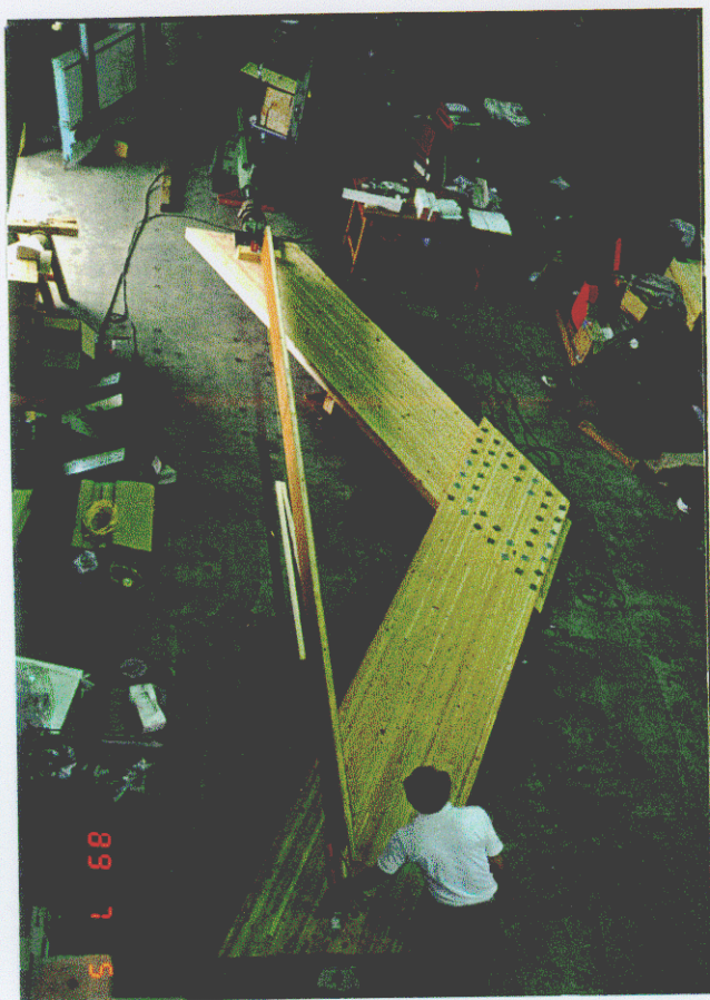
Photo. 10 Static cyclic loading test on a glulam cross lapped knee joint specimen. This moment resisting joint was composed of two column members and a single beam member jointed with 12 mm through bolts with "Appel Rings" inserted at interfaces between beam and column leaves. On-site use elastomer glue was also added for the other specimen (CN5359-15).
