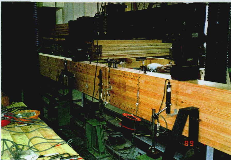
Photo. 7 Four-points bending strength test on glulam beam joint specimen. This joint is basically composed of drift pin joint with insert steel plate, but steel plate itself is also connected on-site by the "high-tension bolts" to make the on-site labor easier than the conventional method (CN9790-14).
