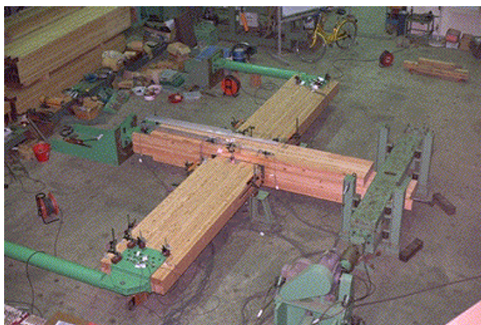
Cyclic loading of Beam to Column Full-sized specimen 実大柱梁十字型接合部の繰返し加力試験
