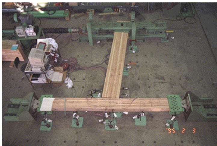
Cyclic loading of Moment-Resisting Full-sized T-shape specimen 実大ト型モーメント抵抗接合部の繰返し加力試験
