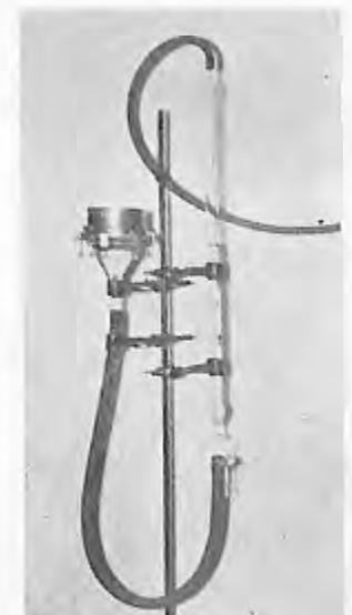
Phot. 1 隔膜吸引法による pF 値測定装置 Apparatus used for measuring the pF values of soil moisture by a vacuume-membrane method
