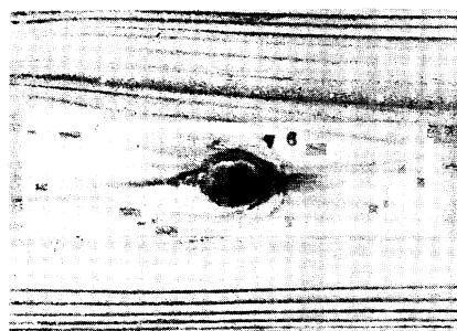
Phot. 5 板目材面における生節の形 Cross-cut section of branch knot on tangential cutting (live-knot portion)
