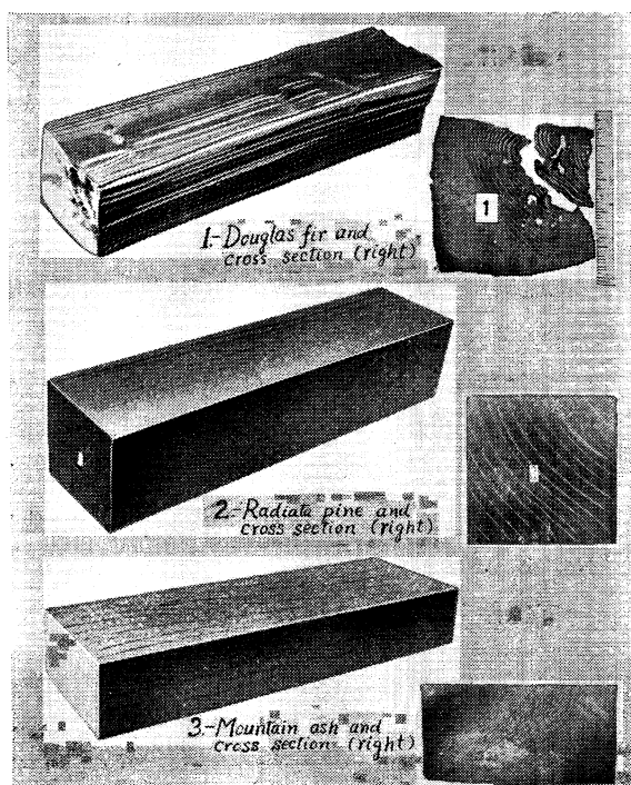
Phot. 3 クレオソート油による高圧処理材 3) ，圧力 70.2 \text{ kg/cm}^2 1時間，油温 59^\circ\text{C} Timber samples treated at 1,000 \text{ lb/in}^2 for 1 hr with a creosote temperature of 138^\circ\text{F} (Transferred from F.P. Newsletter of C.S.I.R.O. 3) )
