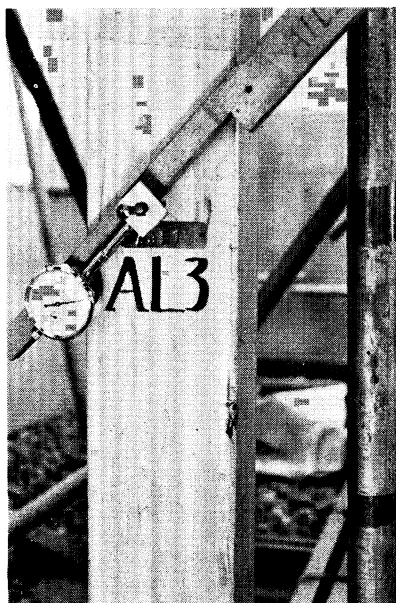
3.6-2 集成材弦長の変形測定法 Measuring method of deformation of chord.
