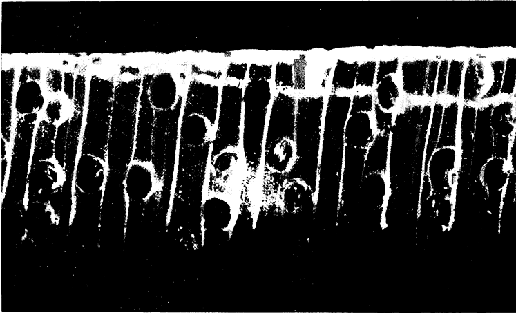
Slight veneer lathe checks (Mark A) Mayapis veneer specimen. No lathe checks are visible. ( \times 50 )
