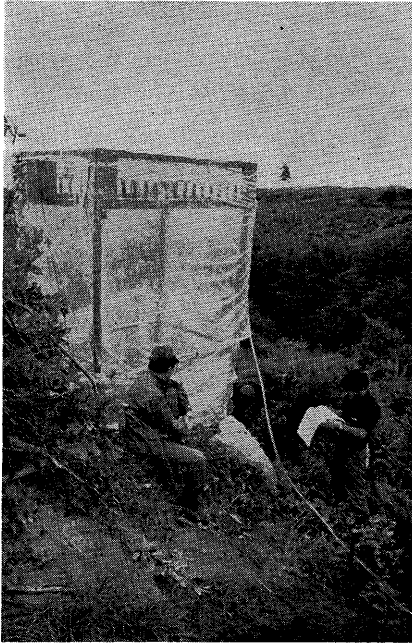
Photo. 8 人工降雨装置を付帯する林試 東北型浸透計 The Rinshi-Tohoku type infiltrometer which has the artificial rainfall apparatus.
