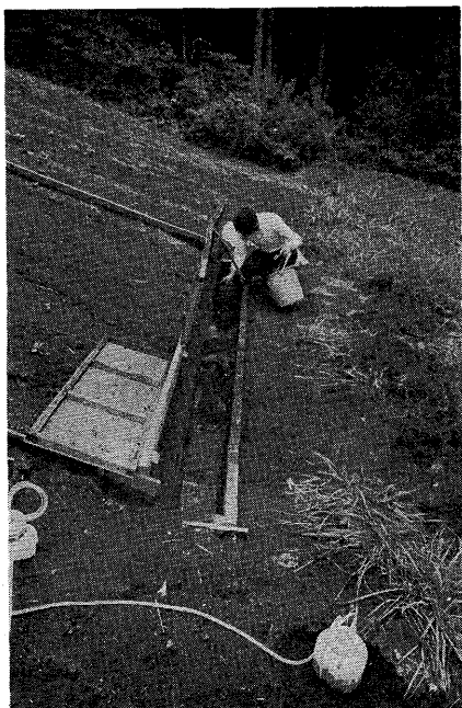
Photo. 4 自然降雨による屋外地表流下区 The outdoor run-off plot which is the object of natural rainfall.
