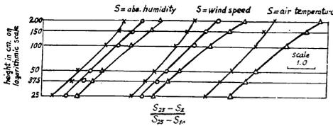
Fig. 6. Vertical profiles of absolute humidity, wind speed and air temperature above short grass.
