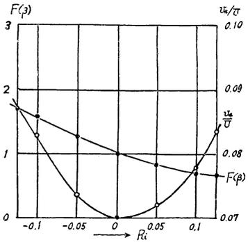
Fig. 9. Relation of  $v_{*i}/U$  and  $F(\beta)$  with  $R_i$ .
