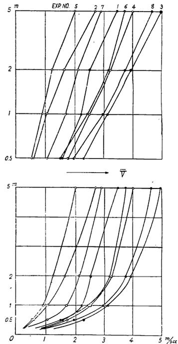
Fig. 10 and 11. Vertical distribution of mean wind velocity.
