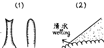
Fig. 5 窪地崩壊 Landslide in the hollow.
