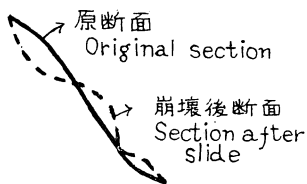
Fig 1. 地圧性崩壊 Slide of landcreep type
