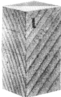
Plate 9. Manner of failure of specimen belonging to Group III—2. ( \alpha=30^\circ , \beta=45^\circ )
