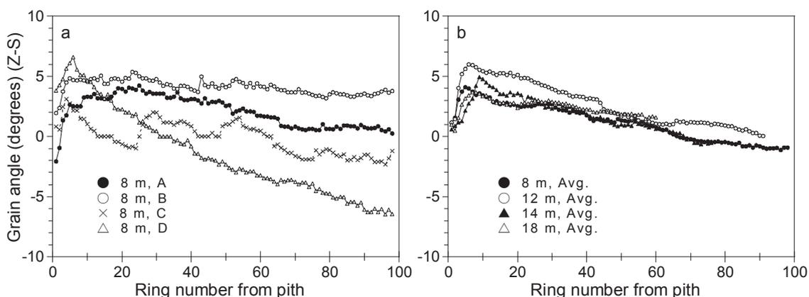
Fig. 2. Radial trend of grain angle. a) Four directions at 8 m above the ground. b) Average of four directions at 8 m, 12 m, 14 m and 18 m above the ground. The minus (Z) grain angle is the deviation to the right of the upper extremity of the longitudinal axis of a tree as viewed by an observer on the ground, and plus (S) grain angle is to the left.
