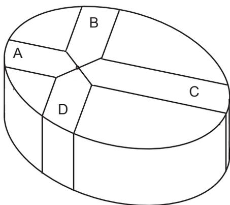
Fig. 1. Directions of the wood property measurements. Two strips (A and C) were taken from the two opposing radii in the direction with the largest diameter. Two strips (B and D) were taken from the two opposing radii in the direction perpendicular to the former strip. The radius was the largest in direction C and the smallest in direction A.
