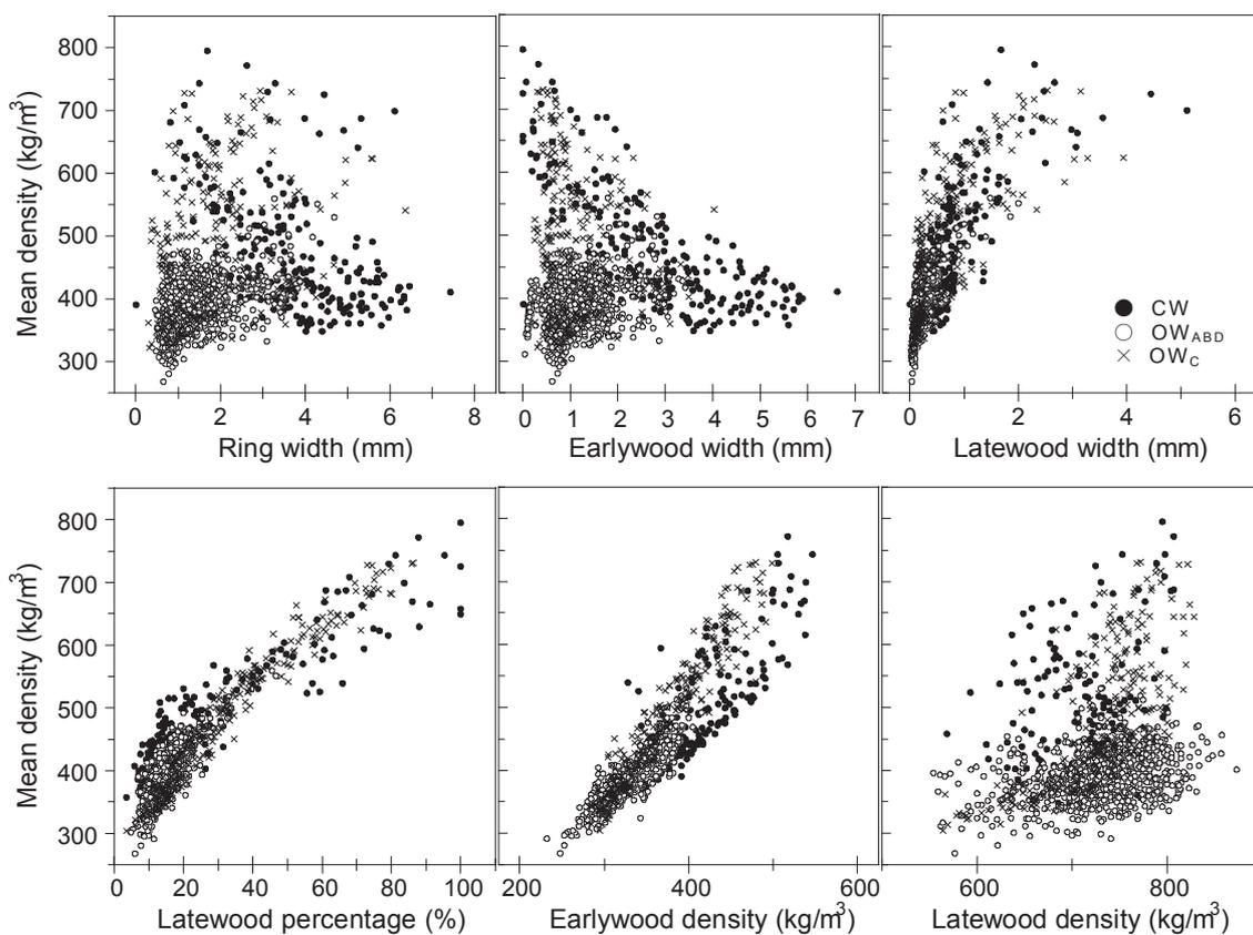
Fig. 5. Relationships between tree ring parameters and mean wood density of the core wood (CW), the outer wood in directions A, B and D (OW<sub>ABD</sub>) and the outer wood in direction C (OW<sub>C</sub>).
