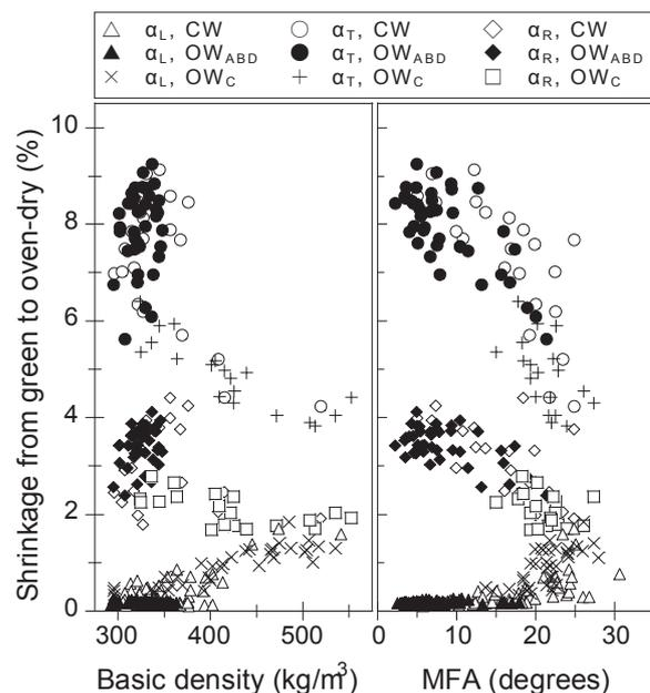
Fig. 7. Relationships between basic density and MFA, and shrinkage of the core wood (CW), the outer wood in directions A, B and D (OW<sub>ABD</sub>) and the outer wood in direction C (OW<sub>C</sub>).
