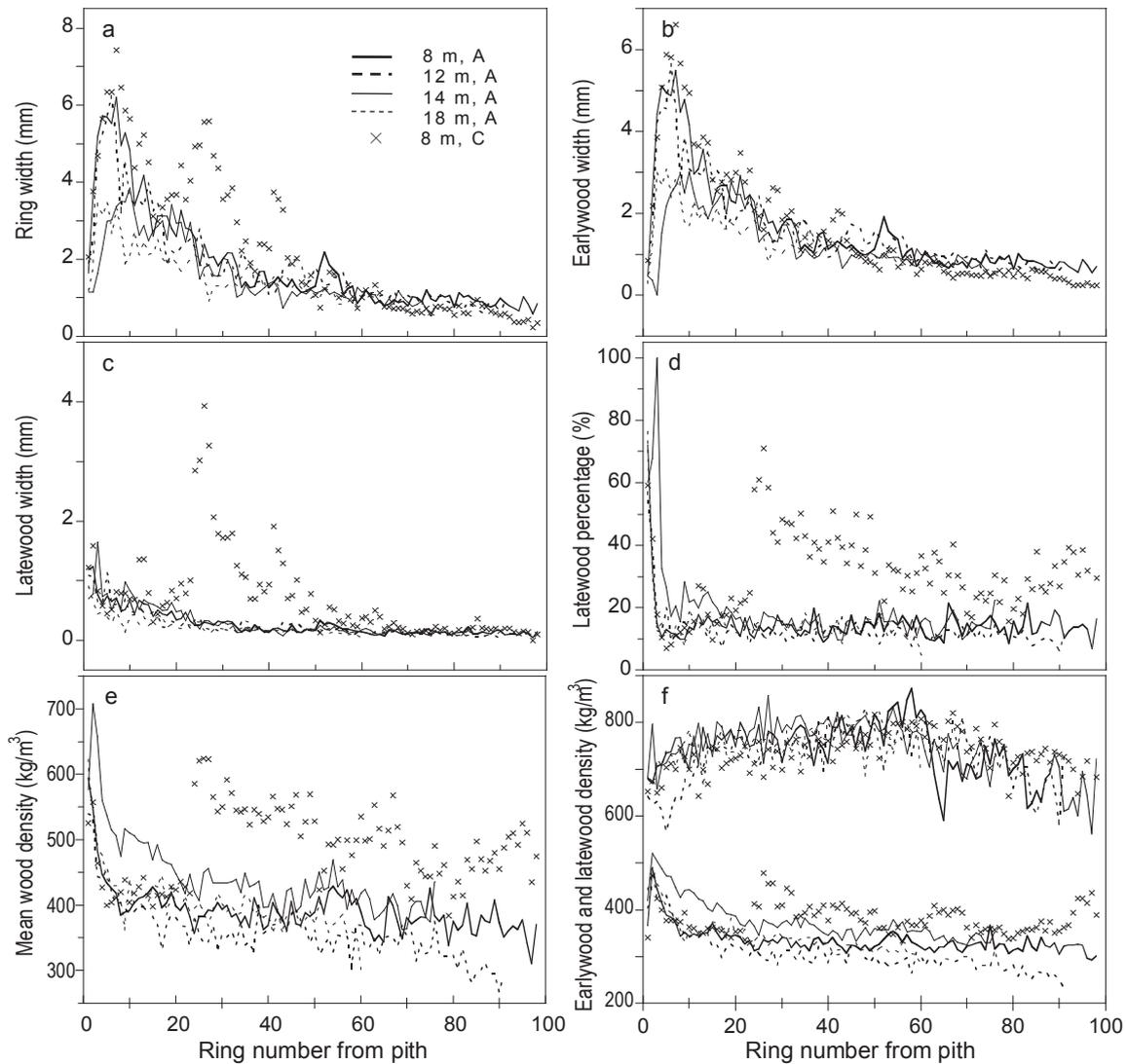
Fig. 4. Radial trends of ring width (a), earlywood width (b), latewood width (c), latewood percentage (d), mean wood density (e) and earlywood and latewood density (f). Direction A at 8 m, 12 m, 14 m and 18 m above the ground, and direction C at 8 m above the ground are shown.
