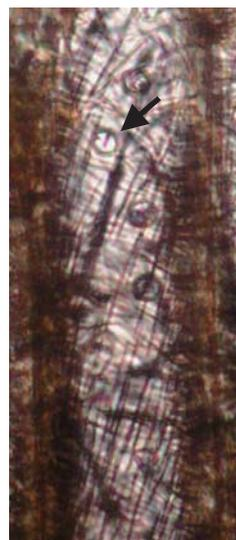
Photo 1. The agreement of the directions between slit-like pit aperture (arrow) and the iodine crystals in a latewood tracheid in *Picea koyamae*.
