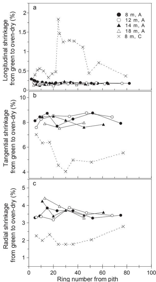
Fig. 6. Radial trends of longitudinal (a), tangential (b) and radial (c) shrinkage. Direction A at 8 m, 12 m, 14 m and 18 m above the ground, and direction C at 8 m above the ground are shown.
