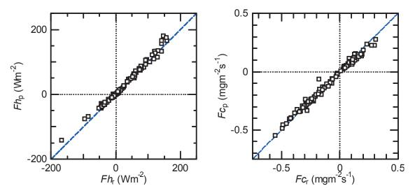
Fig. 3. Correlation diagrams for sensible heat (*Fh*, left) and CO<sub>2</sub> (*Fc*, right) fluxes observed using the portable and routine systems The subscript letter "r" and "p" indicates the value for the routine and portable system, respectively.
