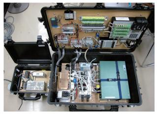
Photo 1. The portable  $CO_2$  flux observation system. Right (main unit): Infrared gas analyzer, air pump, mass flow controller, and solenoid valve are mounted in the lower part; data logger and terminal block are installed on the upper lid part. Left (power unit): Supporting 100–240 V AC and providing 12 or 24 V DC to the main unit through an electric cable.
