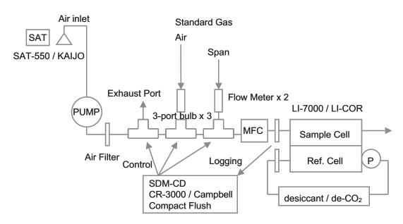
Fig. 1. Block diagram of the portable CO<sub>2</sub> flux observation system. (SAT: sonic anemometer-thermometer, MFC: mass flow controller, P: pump)
