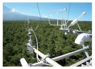
Photo 2. System comparison: SAT and air intake of the portable system (left) and the routine system (right).
