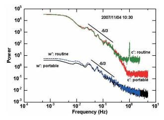
Fig. 2. Fluctuations in the power spectra (before high-frequency correction) of vertical wind velocity (w') and CO<sub>2</sub> concentration (c') for the existing routine and portable systems.
