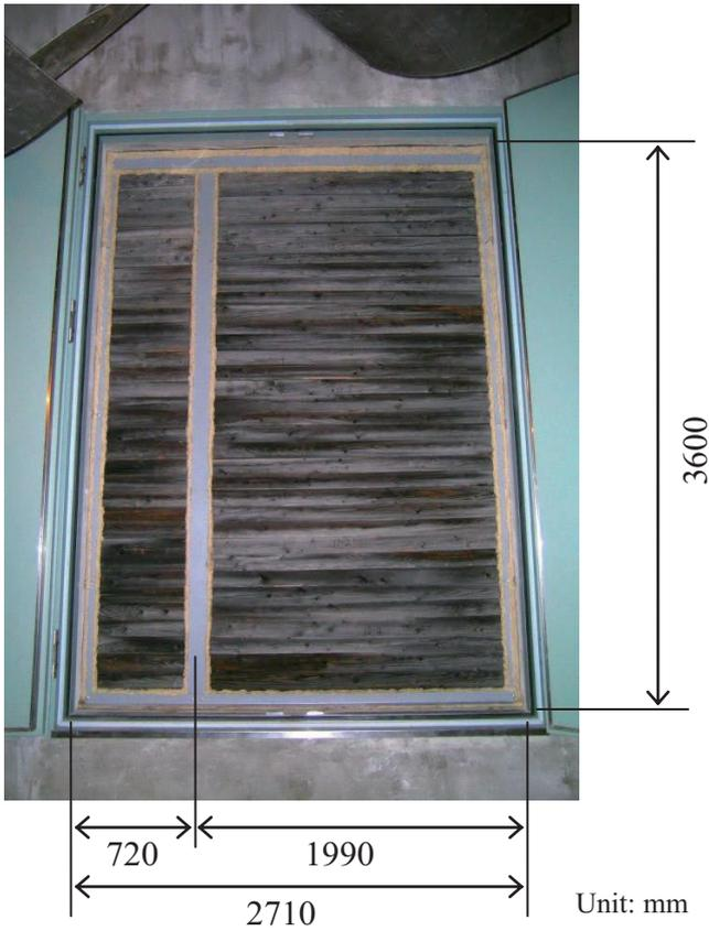
Photo 1 Japanese larch sound barrier without oil clay at the joints.
