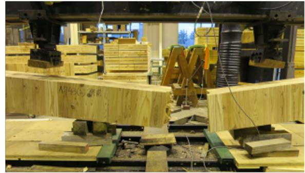
5-layer 7-ply CLT in the minor strength direction
