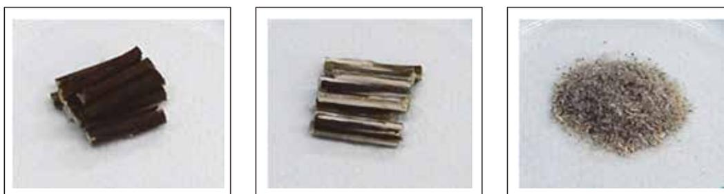
**Fig. 2.** Untreated, crushed, and ground branch samples of 1-2-year-old *Salix* species
