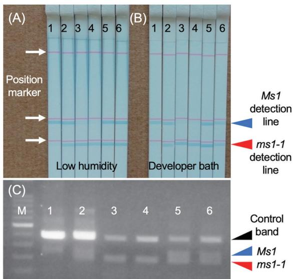
**Fig. 2.** An example of STH-PAS diagnosis for the presence of *Ms1* and *ms1-1* alleles under low humidity condition (A) and developer bath (B) and the result of agarose gel electrophoresis (C). Lane 1: ‘Ōi 7’ (*Ms1/ms1-2*), 2: ‘Suzu 2’ (*Ms1/ms1-1*), 3: SSD-18 (*ms1-1/ms1-1*), 4: SSD-100 (*ms1-1/ms1-1*), 5: FO7-141 (*ms1-1/ms1-2*), 6: FO7-144 (*ms1-1/ms1-2*), M: 100 bp ladder marker.
