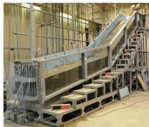
Figure 15. Large-scale experimental equipment to mimic the effect of landslides caused by intensive high rainfall on hillsides. Slide occurs in 2,891 s with heavy rainfall of 100 mm/h.
