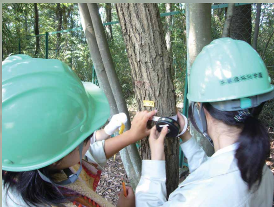
Photo 19. Practice B: Diameter measurement
