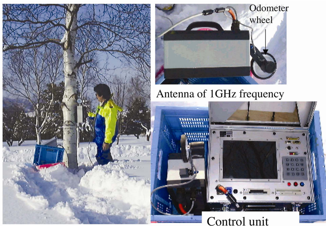
Fig. 2 A portable impulse radar-wave system (ImRa system: Toikka Oy Co. Ltd. Finland) to detect internal information in trunks without destruction of trees.
