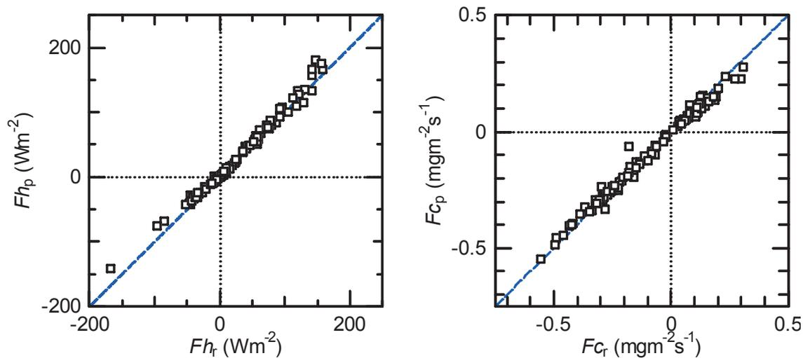
Fig. 3. Correlation diagrams for sensible heat ( $Fh$ , left) and CO<sub>2</sub> ( $Fc$ , right) fluxes observed using the portable and routine systems. The subscript letter “r” and “p” indicates the value for the routine and portable system, respectively.
