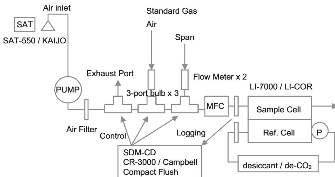
Fig. 1. Block diagram of the portable CO<sub>2</sub> flux observation system.
