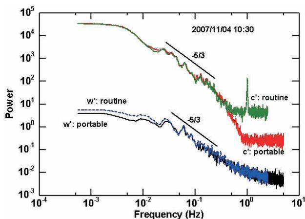
Fig. 2. Fluctuations in the power spectra (before high-frequency correction) of vertical wind velocity ( $w'$ ) and  $\text{CO}_2$  concentration ( $c'$ ) for the existing routine and portable systems.
