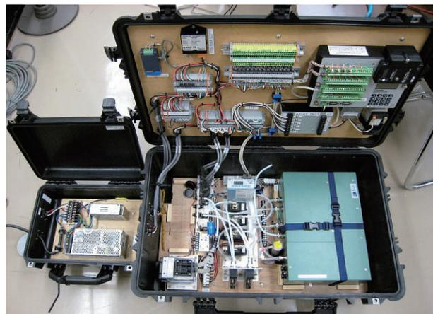
Photo 1. The portable CO<sub>2</sub> flux observation system. Right (main unit): Infrared gas analyzer, air pump, mass flow controller, and solenoid valve are mounted in the lower part; data logger and terminal block are installed on the upper lid part. Left (power unit): Supporting 100–240 V AC and providing 12 or 24 V DC to the main unit through an electric cable.
