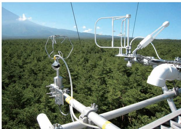
Photo 2. System comparison: SAT and air intake of the portable system (left) and the routine system (right).
